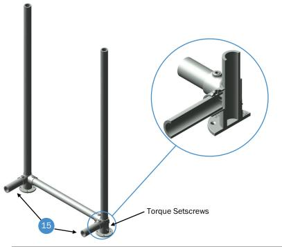
Assembly 5 - Front Legs Torque Setscrews
