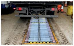
Note A & B Cover is deployed to prevent any fall into the pit. Make a formal weekly check of the condition of the cover.
