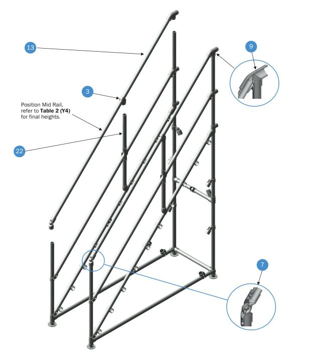
**Assembling the Step** Assembly 10 - Rear Diagonal Assembly
