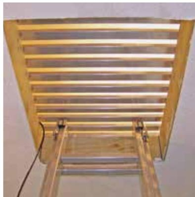
The Loft Hatchway Safety Cover's unique design incorporates folding hollow aluminium slats which hinge to allow access and egress during working. Fixing is by screwing or clamping to the edge of the hatchway while the top side of the slats have anti-slip strips fitted.
