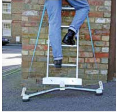
The Anchor Fix is designed to widen the base of a ladder to help stability. It also enables the ladder to be set up on a slope of up to 15° quickly and easily, levelling the base to the optimum position.
