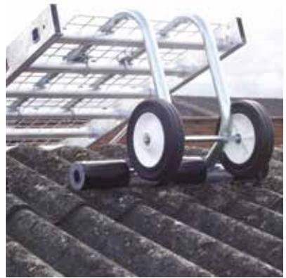
Our Board-Walk system is an open mesh walkway that allows access from eaves to ridge whilst spreading the load on support battens to provide the user with a safer working position. The system is lightweight, easily portable and suitable for fragile roofs.
