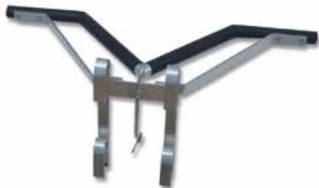
The Ladder Stand Off features a large V which allows the ladder to span around down pipes or rest on corners of buildings. The top of the ladder is kept 330mm off the wall making it ideal for use when working under eaves.
