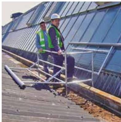
Our Valley-Walk system is a mobile walking frame for one or two persons, designed to aid access along valley gutters and to provide mobile roof cover. Easy to transport and assemble, the unit features cushioned outriggers for comfort which are filled with safety mesh. The Valley-Walk is suitable for typical symmetrical valleys and can be adjusted to suit asymmetrical designs such as northern lights.
