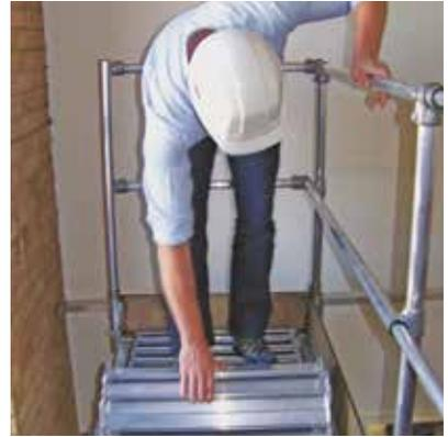
Walk Thru Stairwell Access has been designed as a safe solution to stairwell maintenance which is traditionally undertaken using boards and step ladders. The system provides users with a stable working platform above a staircase, whilst still allowing access up the stairs to the first floor. This is achieved by simply rolling back the aluminium slatted decking as required.
