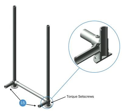
Assembly 5 - Front Legs Torque Setscrews
