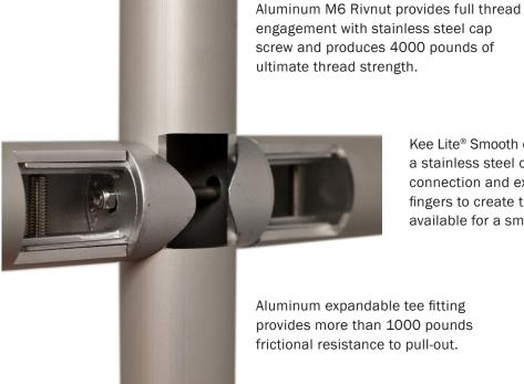
Kee Lite® Smooth components utilize a stainless steel cap screw for thru-bolt connection and expanding internal fingers to create the most rigid connection available for a smooth handrail system.
