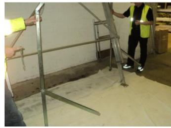
Position the back Legs by removing the middle pin first, holding onto it and lowering the brace.
