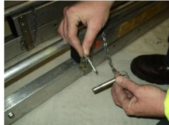
Pull out the clips and release the two Cross Braces from their stored position.
