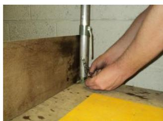
Secure all the uprights in the locating sockets with the pins and 'R' Clips provided.
