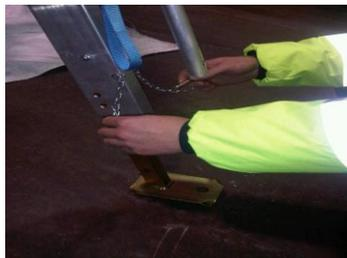
The Feet maybe adjusted in 1.2in (30mm) increments but in extreme cases either Leg can be adjusted Independently. Insert Pin and 'R' Clip to secure.
