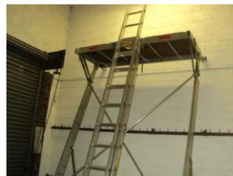
The Ladder is placed against the Platform, extended 3 feet (approximately 1 meter) above platform level between the Tie in Lugs of the Platform and shifted to the right to allow room to the left between ladder and gate.
