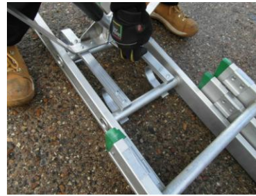
Position the ladder stand-off over the top end of the ladder ensuring the hooks are pushed firmly over the rungs.
