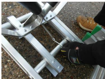
Pull the spring hook over the second rung ensuring it's firmly secured into position. WARNING! It is very important this spring hook is fixed into position before use, as it prevents the Ladder stand-off sliding off the top end of the Ladder.
