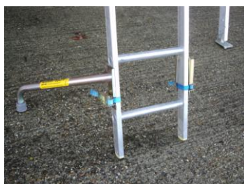
Use Ladder spurs supplied by Easi-Dec to aid stability and prevent outward slip.
